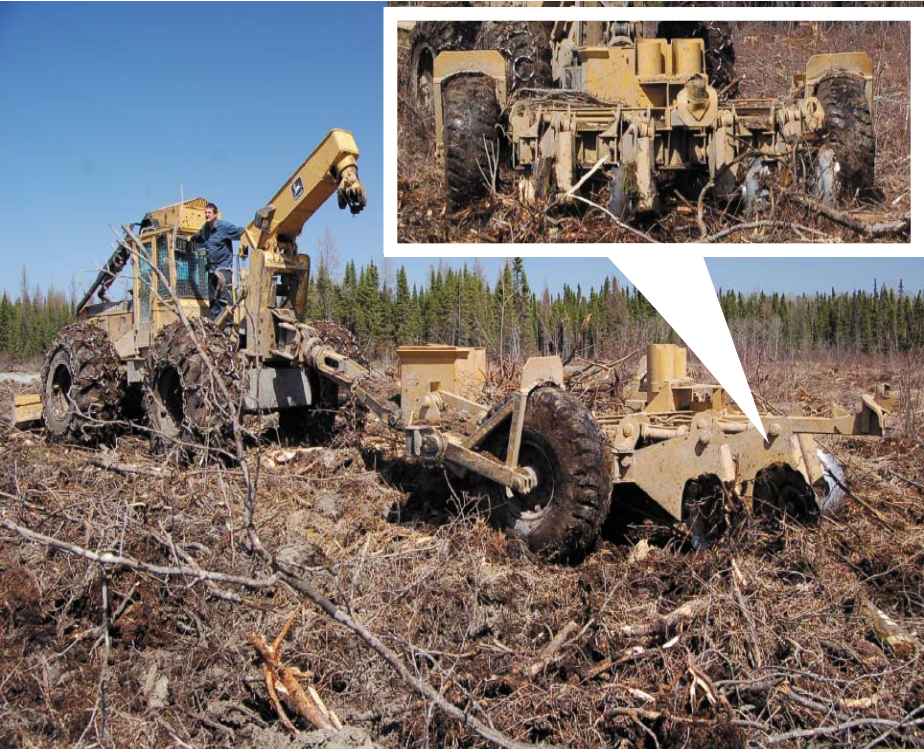
1- Harrow (slicing the top soil) - break up and spread the debris
