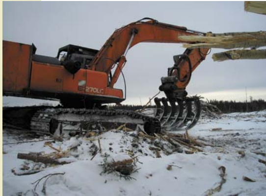
Making piles with tree ends and branches
