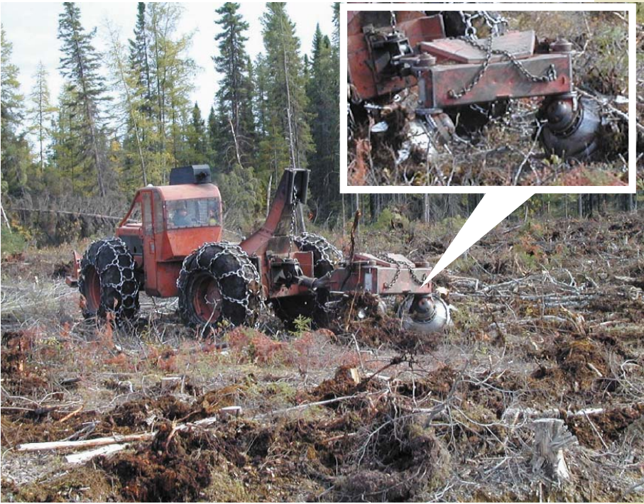
1- Serrated discs scratching the top soil. - Doesn't break the debris
