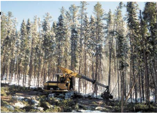
Cutting the trees, taking out the branches and making 2.4 to 4.8 meters logs
