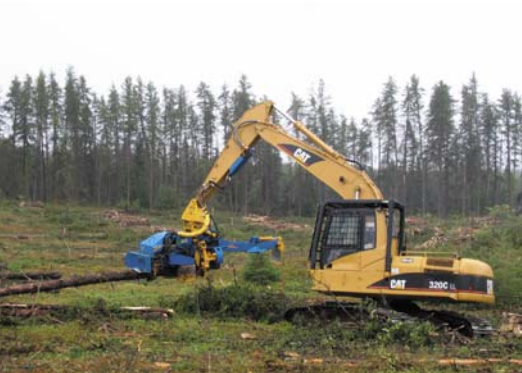
-Taking but the branches -Making 2.4 to 4.8 meters logs
